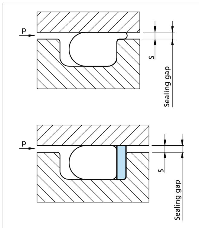
Figure 3 O-Ring installation with and without Back-up Ring
