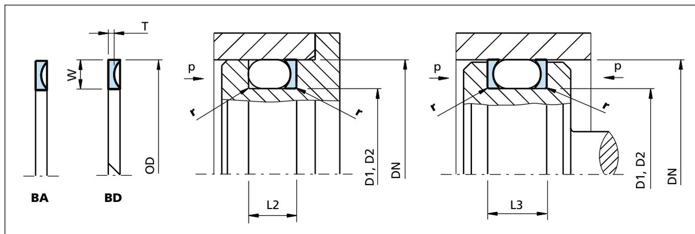
Figure 7 Installation drawing
