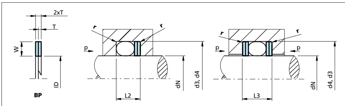
Figure 11 Installation drawing
